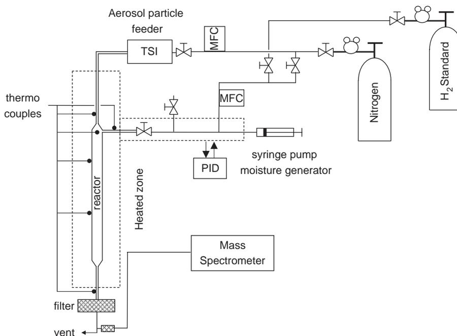
Fig. 1 – Schematic of the aerosol flow reactor setup.
