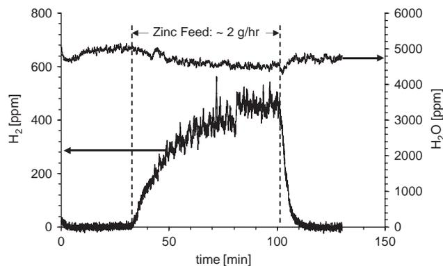
**Fig. 8** –  $\text{H}_2$  and  $\text{H}_2\text{O}$  concentration in flow reactor effluent during hydrolysis of nano-sized zinc powder at  $\sim 703 \text{ K}$ , a particle feed rate of  $\sim 2 \text{ g/h}$  and a gas flow rate of  $7 \text{ l(STP)/min}$  ( $5.21 \text{ mmol/s}$ ).
