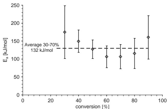
**Fig. 7** – Activation energy as function of conversion determined by isoconversion method from data in Fig. 6.
