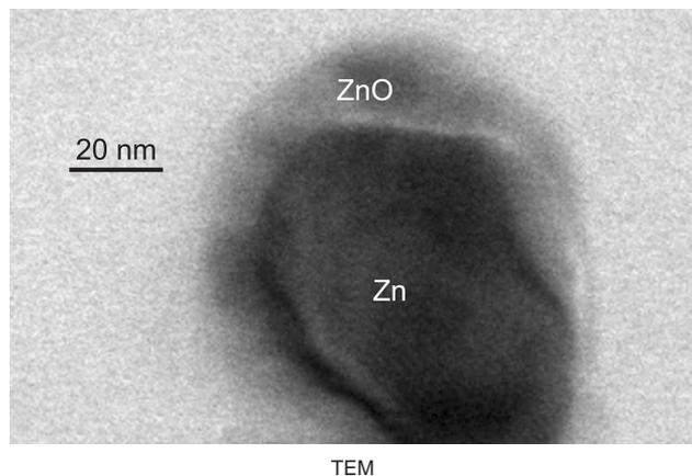
Fig. 9 – TEM image of nano-zinc reacted at 733 K.
