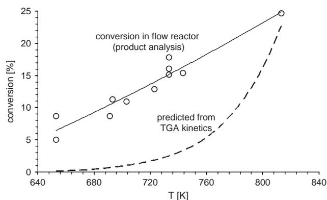
Fig. 10 – Measured and predicted conversions of nano-sized zinc powder in the aerosol flow reactor.
