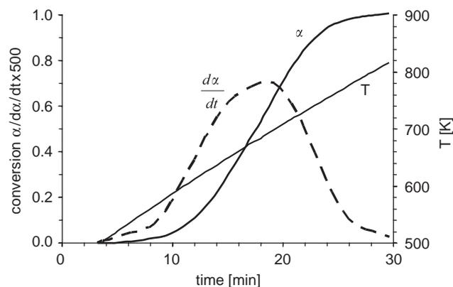
Fig. 3 – Hydrolysis of 54.9 mg nano-sized zinc powder at a heating rate of 11.9 K/min and a water concentration of 1.5 vol% in the TGA—sample dispersed on quartz wool in wire mesh crucible.
