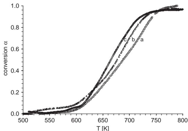
**Fig. 6 – Hydrolysis of three samples of about 20 mg dispersed on quartz wool in a wire mesh cage at different heating rates and a water concentration of 1.5 vol%: (a) 5.3 K/min (23.3 mg); (b) 9 K/min (25.9 mg) and (c) 12.3 K/min (19.5 mg).**
