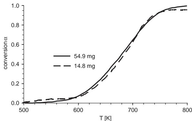
Fig. 4 – TGA measurements with 14.8 and 54.9 mg samples at a heating rate of 11.9 K/min.
