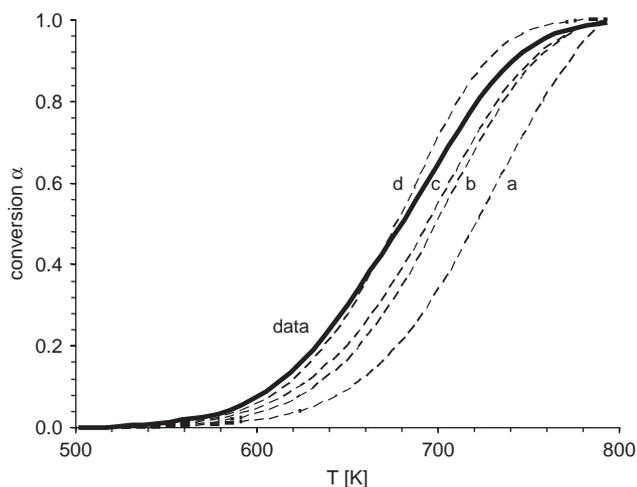
**Fig. 5 – Comparison of experimental data from Fig. 3 with predictions using different reaction models  $f(\alpha)$ : (a)  $3(1 - \alpha)^{2/3}$ ; (b)  $3(1 - \alpha)^{2/3} + 2(1 - \alpha)$ ; (c):  $(1 - \alpha)^n$ ,  $n = 0.4$  and (d)  $(1 - \alpha)^n$ ,  $n = 1.6$ .**
