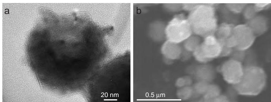
Fig. 2 – Images of nano-sized zinc powder: (a) TEM and (b) SEM.
