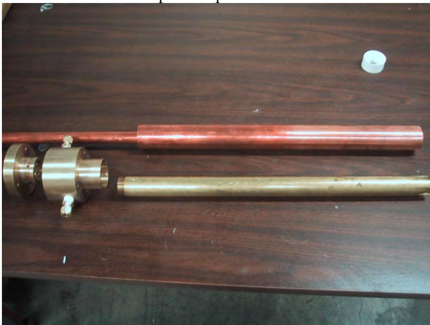
Figure 4: Disassembled quench tube
