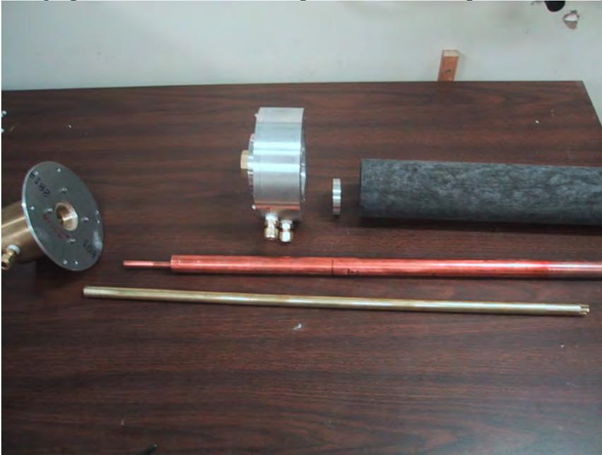
Figure 2: Lance exploded view
