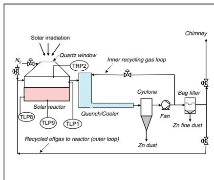
Figure 3: Flow diagram of SOLZINC solar chemical pilot plant: solar concentrating system, solar reactor, off-gas system, and diagnostic instrumentation.
