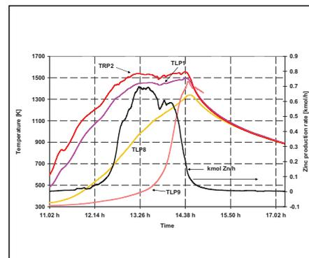
Figure 4: Temperatures and production rate during a typical test (experiment C in table). TRP2: partition plates; TLP1: reaction chamber; TLP8: SiC lateral wall; TLP9: SiC bottom plate.
