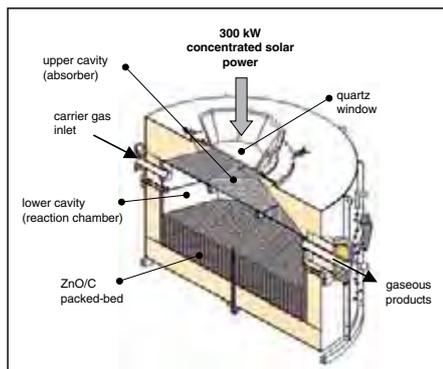
Figure 2: Schematic of the 300 kW solar chemical reactor: solar absorber (upper cavity) and reaction chamber containing a ZnO-C packed bed (lower cavity) [1].
